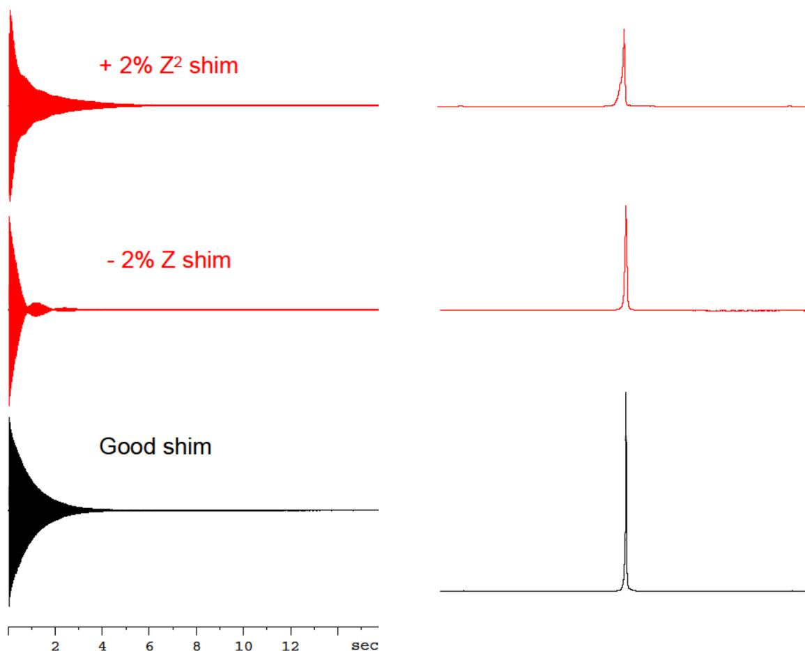
Figure 2.1. Effect of shim current changes on FIDs and spectral lines. Data acquired on a Bruker Avance 500 Spectrometer.  $^1\text{H}$  NMR of 3%  $\text{CHCl}_3$  in acetone- $d_6$ .
